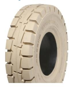
140/55-9 (15X5.5-9,15X5 1/2-9) 4.00E STARCO TUSKER EASYFIT NON MARKING 114A5/104A5 15x5.5-9,15x5 1/2-9
